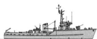
424t, 46.4x8.6x2.5m, 2gg,2gt or 2d, 2000hp, 15kts, 38p; 1x1-40/60, 1x1-20/70, mechanical, acoustic, magnetic sweeping gear; radar
